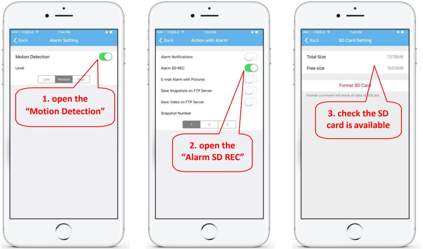
Motion detection alarm recording is recommended when the Micro SD card is small.
