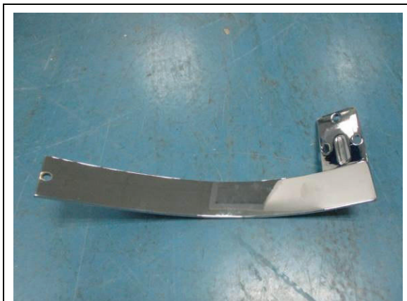
Sample #1 before salt spray tests - View 1
