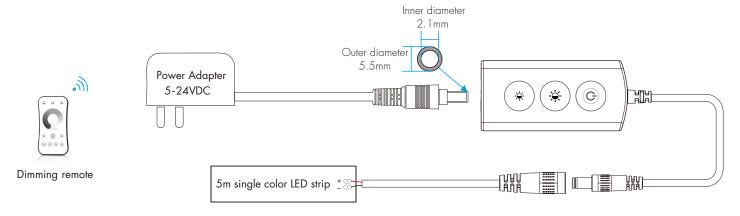
Note: Press and hold the (\*) and (\*) (Brightness-) button for 2s, output LED flashes 3 times, the light on/off fade time will change between 3s and 0.5s.
