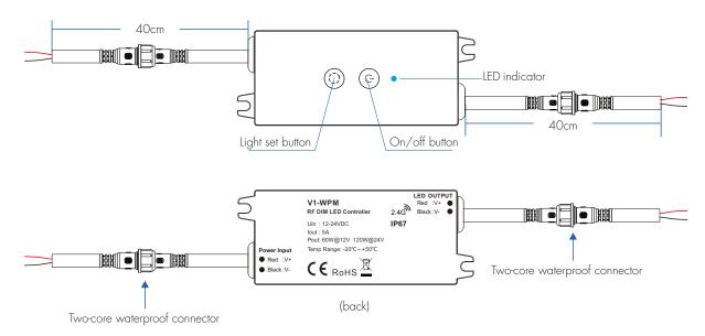
NOTE: When installing, align the insert and tighten the nut.
