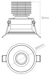
Install hole size: Ø70mm
