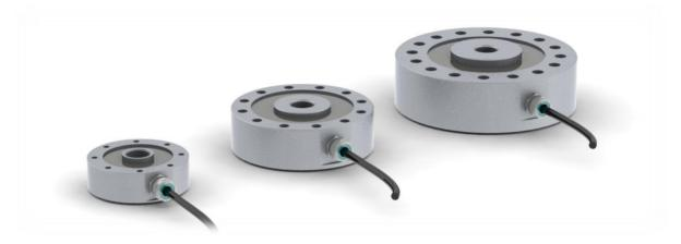
Custom Pancake Load Cells are strain gauge based transducers with temperature compensation and excellent overall performance. This type measures tensile and compressive loads up to 140kN with better than ±0.1% non-linearity. Covers are fully welded and rated to IP67.
